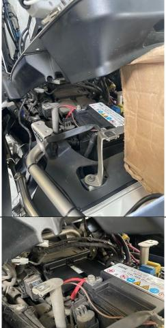
Secure the LVD Power Timer to the top of the BCA case with the leads facing the auxiliary battery.
